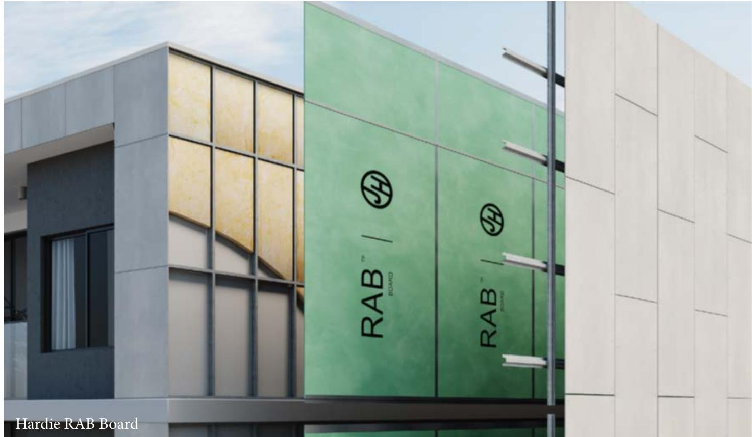
RAB™ Board is a 6mm specialised fibre cement rigid air barrier that can be used beneath façade systems and external claddings, providing added protection against the elements.
